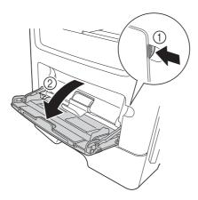
Pull out the extension guide of the Manual Feed Tray.
